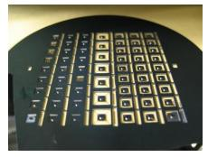
Ex. Capacitive 3-axis accelerometer
