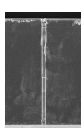
60μm Diameter Via Hole etched to a depth of 200μm
