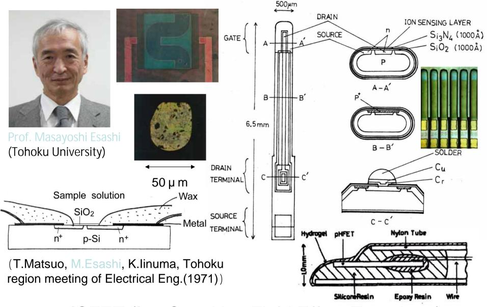
ISFET (Ion Sensitive Field Effect Transistor) (wafer process for reliable assembly) (M.Esashi & T.Matsuo, Supplement to the J.J.A.P.,44 (1975) 339) PR-1165
