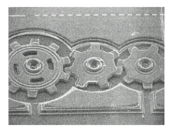
(K. J. Gabriel, W. S. N. Trimmer and M. Mehregany, "Micro gears and turbines etched from silicon", in Tech. Digest of the 4<sup>th</sup> Int. Conf. On Sold-State Sensors and Actuators (Transducers '87, Tokyo, June 1987), pp. 853-856)
